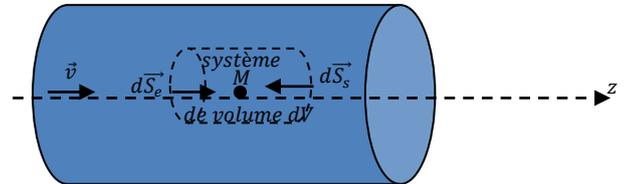
$$\begin{aligned} dm(M, t + dt) - dm(M, t) &= j_z(x, y, z, t)dS_e dt \\ &\quad - j_z(x, y, z + dz, t)dS_s dt \end{aligned}$$
